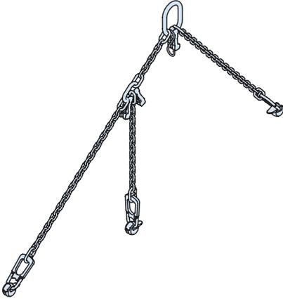
The DEHA Pipe installation device can be described as being a lifting-device as well as an installation device. It can be used directly as a load lifting device or as a hoisting gear. It consists of 3 chain lengths, with a DEHA Universal-head lifting link attached at each of the 3 ends. A symmetrical or an asymmetrical hoist configuration is possible:
